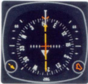
1. Approaching the STL VORTAC, the controller asks you to hold Southwest of the VORTAC on the 244° radial, right turns. You are now over the station with a 064° course selected (the TO/FROM indicator has swung to "FROM"). (Set your Heading Bug to the reciprocal...or outbound heading...244° for easy reference and begin your right-turn holding pattern.)
