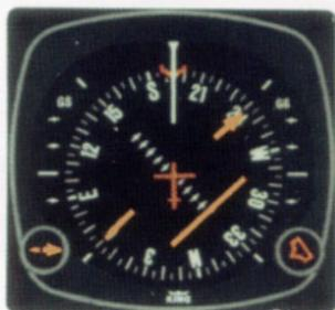
2. During the procedure turn outbound, the deviation bar shows pictorially that the aircraft (as represented by the symbolic aircraft in the center of the KI 525A) is flying away from the Localizer centerline at 45° angle when the heading marker is under the Lubber Line. Note that left-right deviations of the course bar give "fly-to" indicators, just as on the front course.
