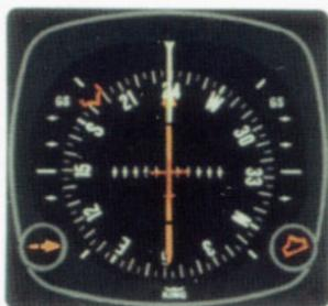
1. You are outbound on the back Localizer course, having already set the Selected Course pointer to the inbound front course at 238°. The Heading Bug is preset at 193° for the procedure turn. (Since there is usually no Glideslope signal on a back course, the Glideslope pointers are out of sight.)
