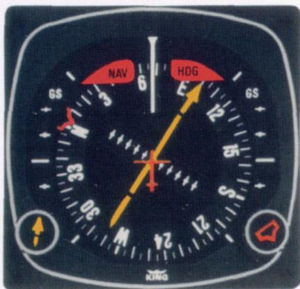
The KI 525A Pictorial Navigation Indicator is the panel display for the KCS 55A compass system. By combining the display functions of the standard Directional Gyro, the VOR and LOC deviation indicator with Glideslope display, the KI 525A simplifies navigation and reduces cockpit workload.
